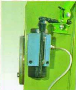
Centralized Lubrication Pump
